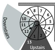
If the first step from the bottom is not accessible, try, if possible, to move the arrival point, to reverse the direction of ascent or to add or remove steps.
